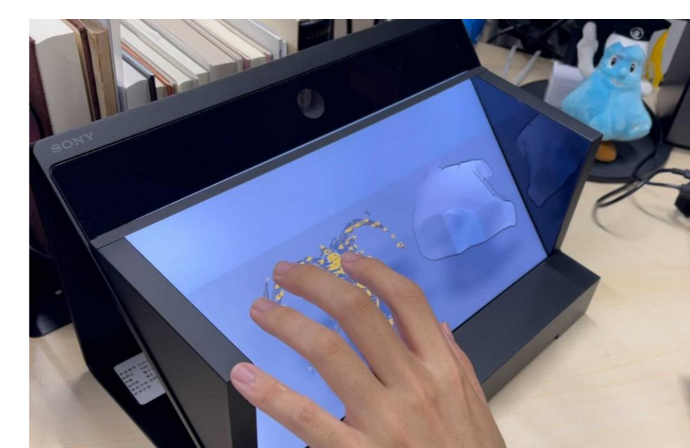
Fig6. The 3D image displayed on the spatial reproduction display and motion capture captured hand movement
