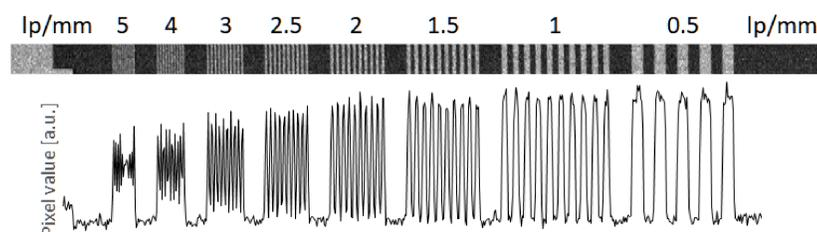
Fig. 2. Imaging result of an X-ray test chart that includes 0.5–5 lp/mm line pairs. The bottom graph shows the averaged line profile
