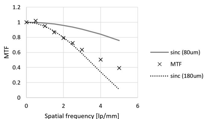
Fig. 3. Calculated MTF based on the X-ray test chart results. The solid line denotes the sinc function corresponding to an MTF of 80 $\mu$ m sampling, the cross-marks denote the measured MTF of the proposed imager, and the dashed line denotes the sinc function corresponding to an MTF of 180 $\mu$ m sampling
