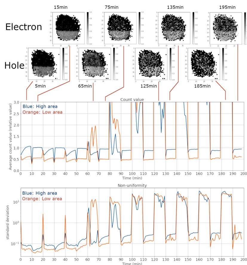
Fig. 4. The upper graph shows the change over time in the count value. The bottom graph shows the standard deviation of the counts per pixel. Larger values indicate poor pixel-by-pixel uniformity. The blue line is the unshielded area and the orange line is the shielded area.
