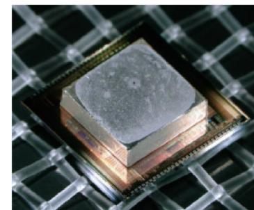
Fig. 1. Structure of the assembled TlBr X-ray imager (left) and the structure after stacking (right)
