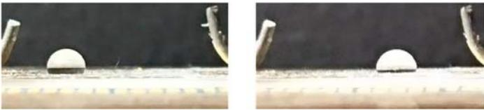
Fig. 4. Droplet manipulation on SLIPS. (a) before and (b) after transportation
