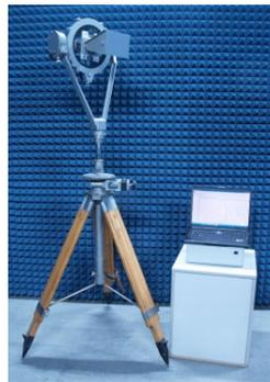
Fig. 5. Anechoic chamber with a control unit of the YUST FarField hardware and software complex with a laptop, as well as a rotary support with an antenna P6-126
