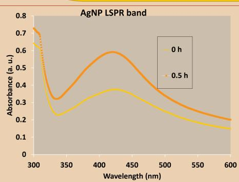
Fig 7. AgNP suspension absorption spectrum before and after UV C radiation exposure
