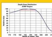
Fig 4. Set of Spread Out Bragg Peaks
