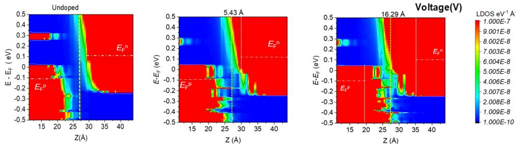
Local Density of States (LDOS) interpretation for  $V_{bias}=0.2$  V. D-A pair makes the tunnel barrier narrower, depending on the configuration of the donor-acceptor pair
