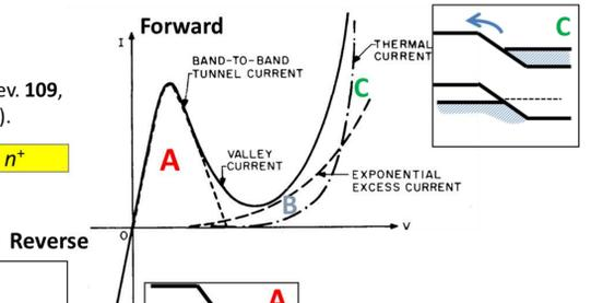
Basic behavior of a tunnel diode can be reproduced:
